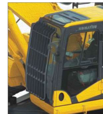
Cab front full height guard level 2 (ISO 10262)
