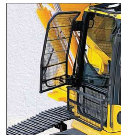
Cab front full height guard level 1 (ISO 10262)
