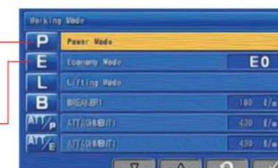
Boom pushing force is increased, ditch digging and box digging operation on hard ground are improved.
