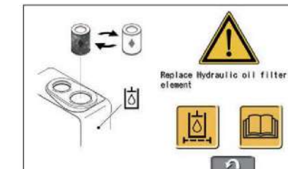
Clogging hydraulic oil filter caution
